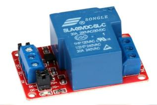
The Single-channel 5V 30A Relay Module power failure relay is a 1-channel relay module board with LED indicators, It can be controlled by microcontrollers such as Arduino, AVR, PIC, ARM any other microcontroller operating at 5V.
